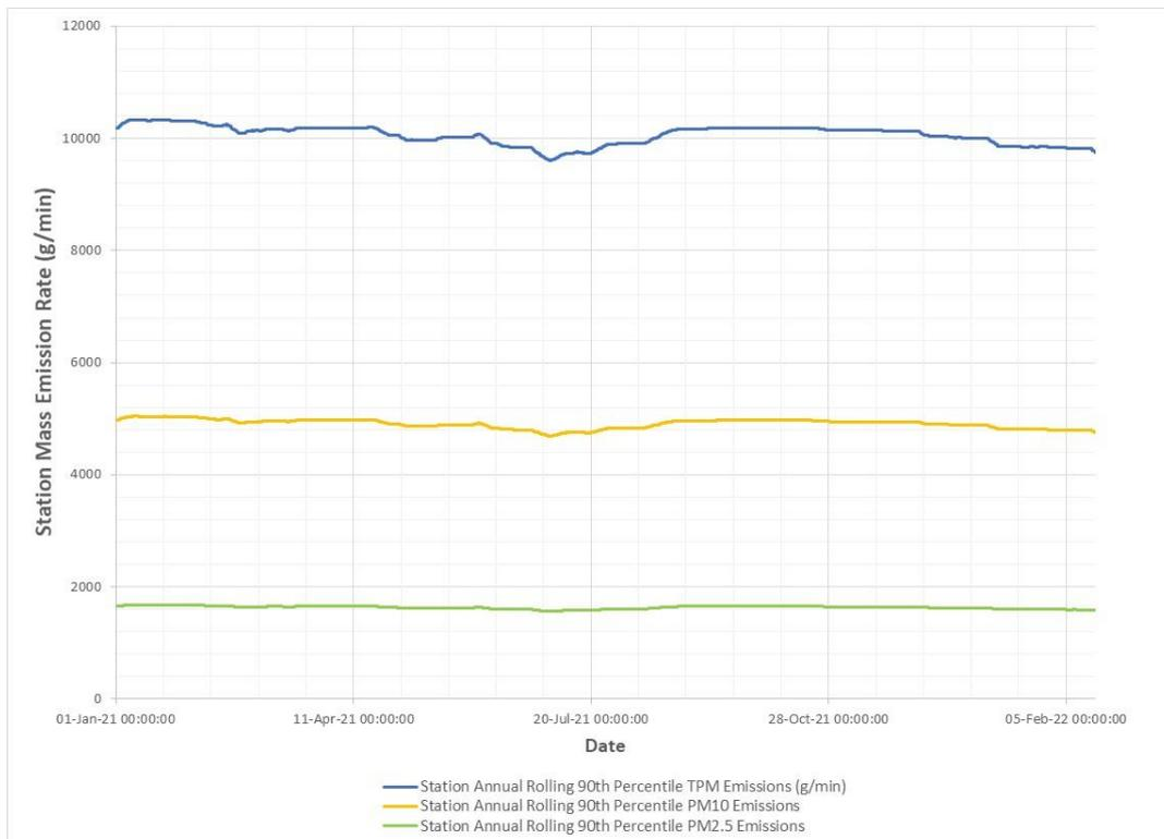
**Figure 1: Example Annual Rolling 90<sup>th</sup> Percentile Emission Rates for Station TPM (continuously monitored) and PM<sub>10</sub> and PM<sub>2.5</sub> estimated using correlations with TPM**
