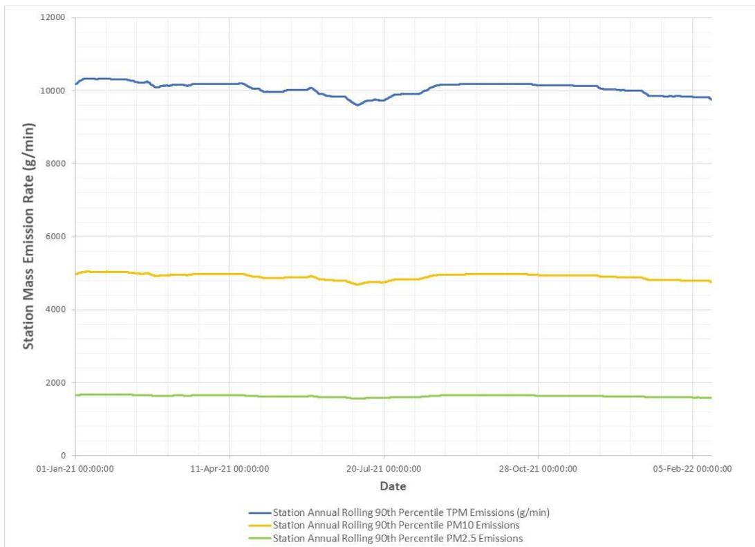
**Figure 4: Example Annual Rolling 90<sup>th</sup> Percentile Emission Rates for Station TPM (continuously monitored) and PM<sub>10</sub> and PM<sub>2.5</sub> estimated using correlations with TPM**
