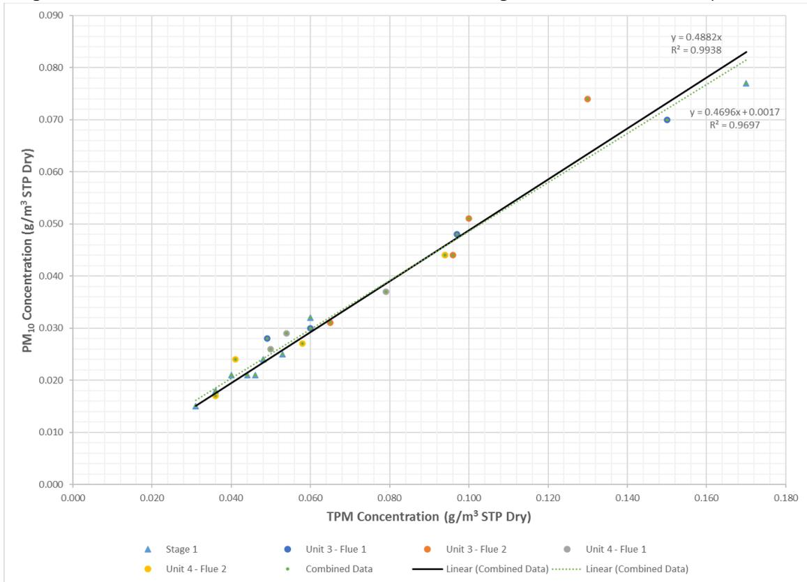
**Figure 2: PM<sub>10</sub> to TPM correlation with all Stage 1, Unit 3 and Unit 4 Test Data (Jun 21 – Feb 22)**
