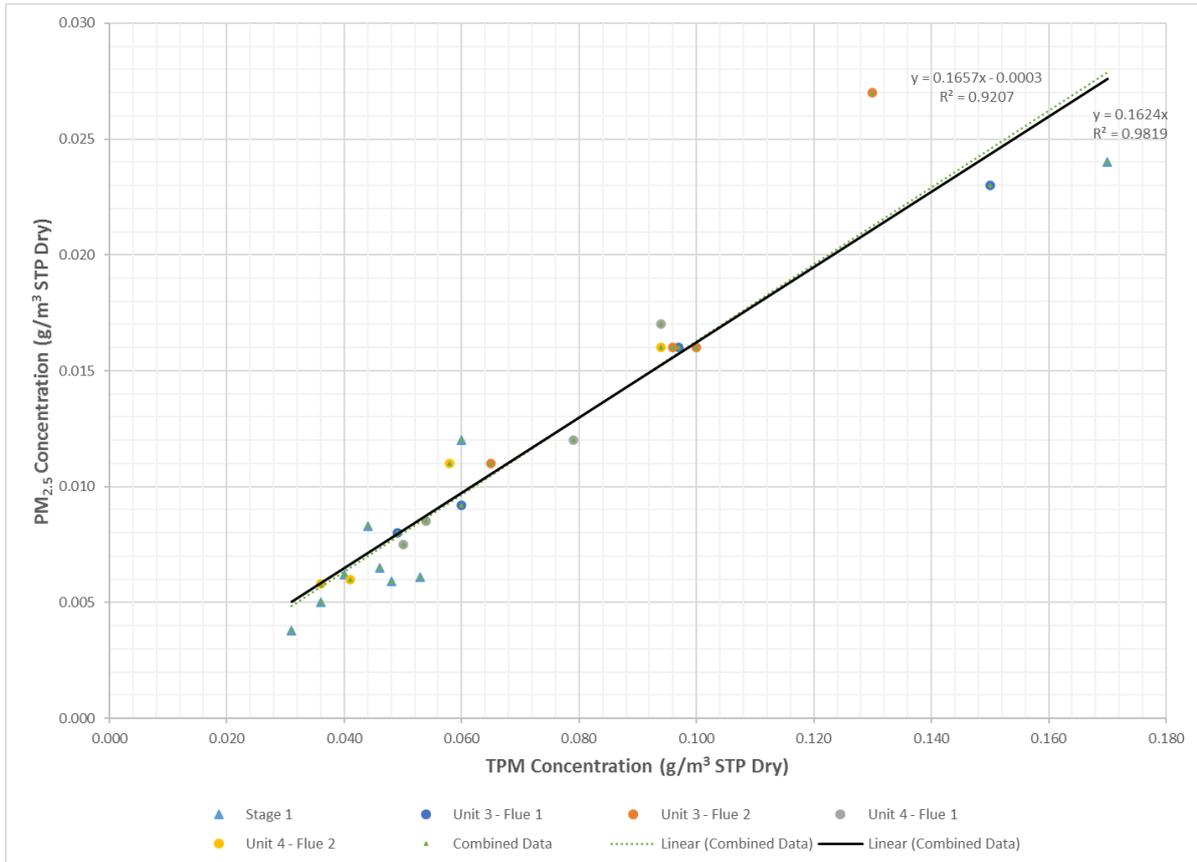
**Figure 3: PM<sub>2.5</sub> to TPM correlation with all Stage 1, Unit 3 and Unit 4 Test Data (Jun 21 – Feb 22)**
