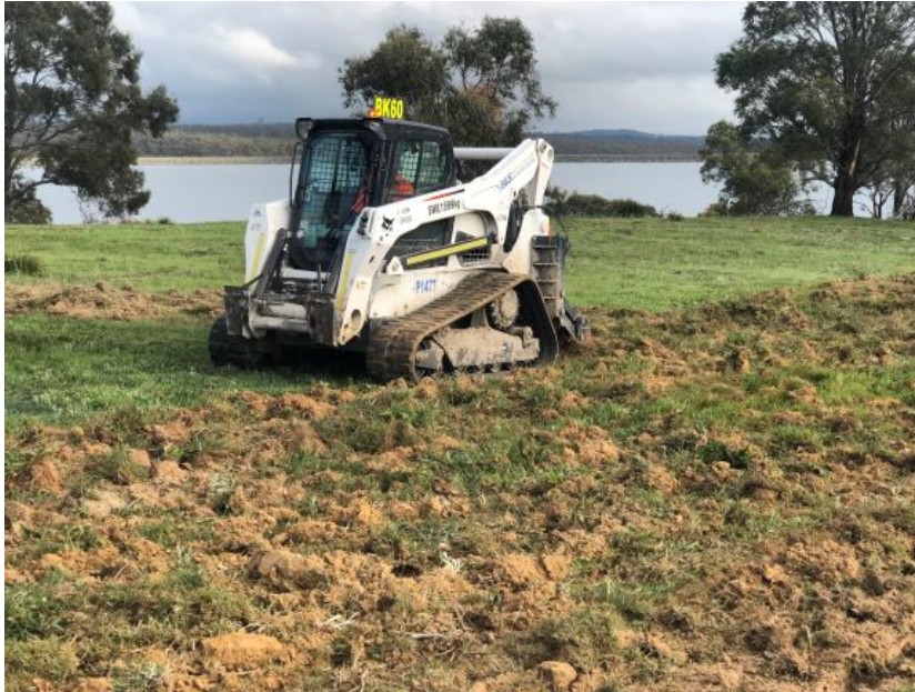
Plate 2. Bobcat Positrack fitted with rear ripper tines creating a seed bed at the BOA.
