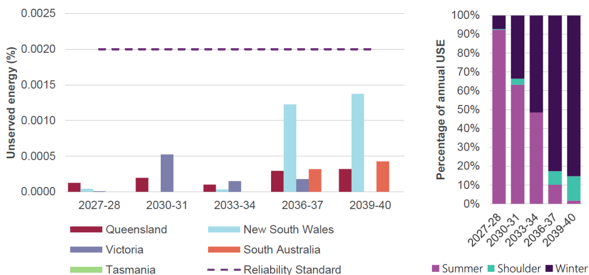
Figure 9 Forecast expected unserved energy in Step Change Scenario (left) and seasonal share of NEM-wide reliability events (right)
