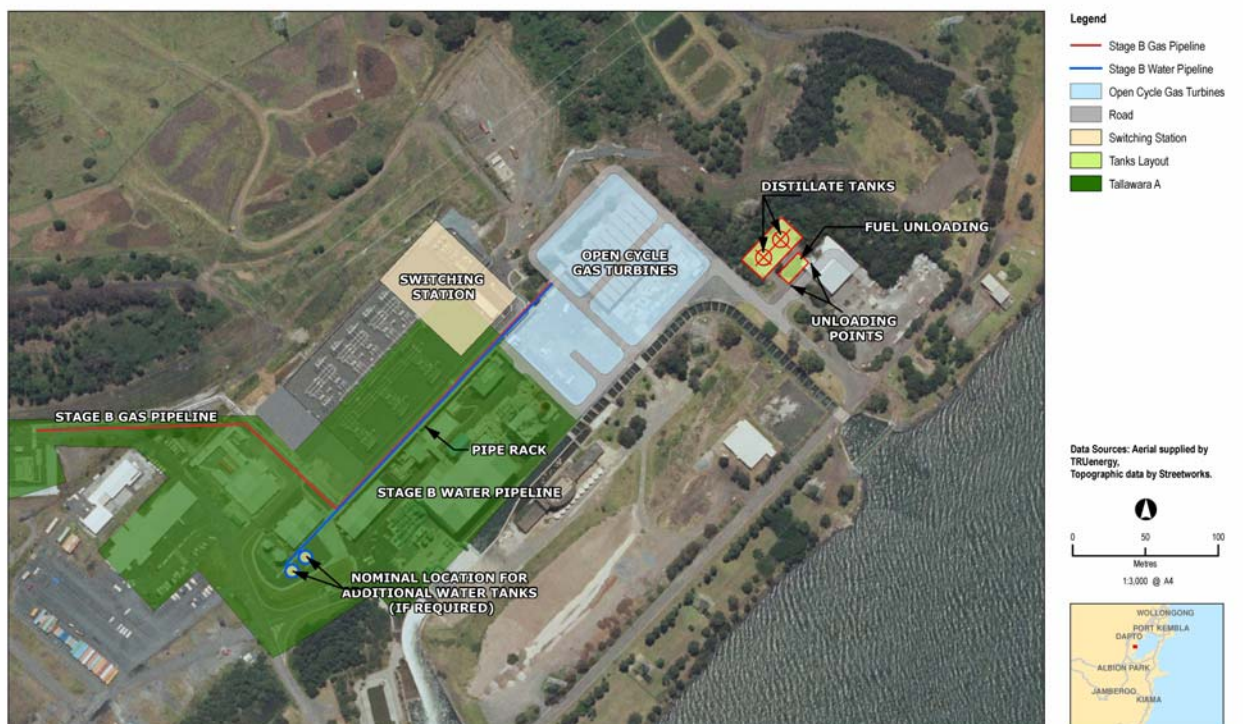
Figure 6 – Tallawarra Stage B General Site Layout, Open Cycle Gas Turbine Power Station (SKM/TRUenergy, 2009)
