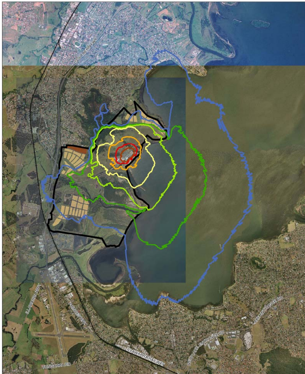
Figure 11: Noise Contours for Tallawarra Stages A and B Combined Cycle Power Stations Operating Under Adverse Meteorological Conditions (SKM/TRUenergy, 2009)
