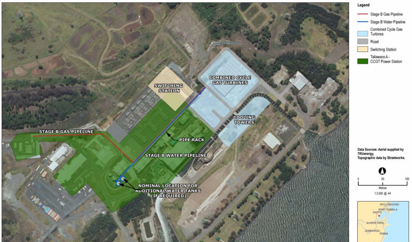
Figure 7 – Tallawarra Stage B General Site Layout, Combined Cycle Gas Turbine Power Station (SKM/TRUenergy, 2009)
