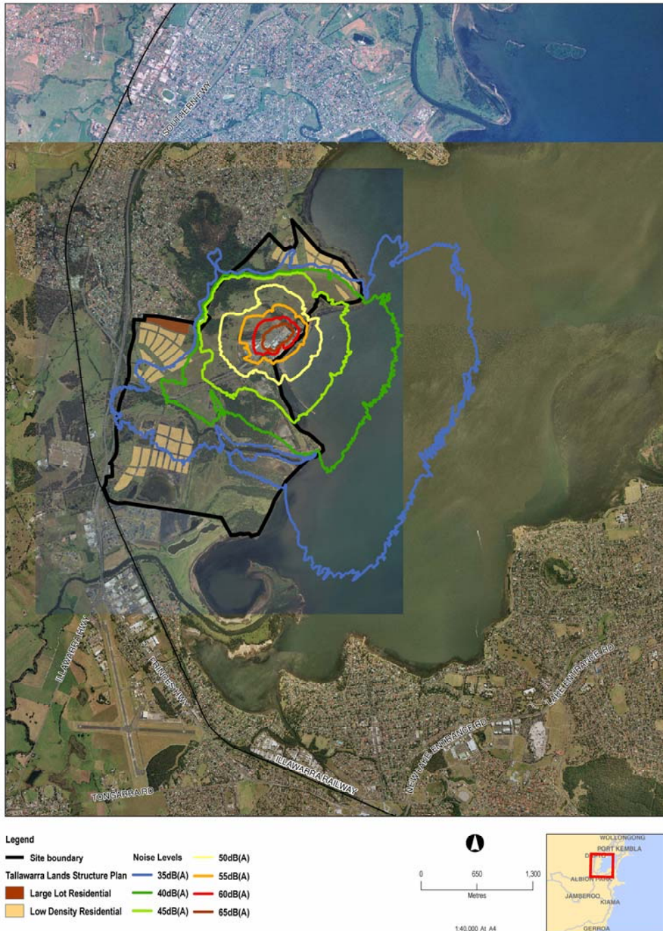
Figure 12: Noise Contours for Tallawarra Stage A Combined Cycle Power Station and Stage B Open Cycle Power Station Operating Under Adverse Meteorological Conditions (SKM/TRUenergy, 2009)
