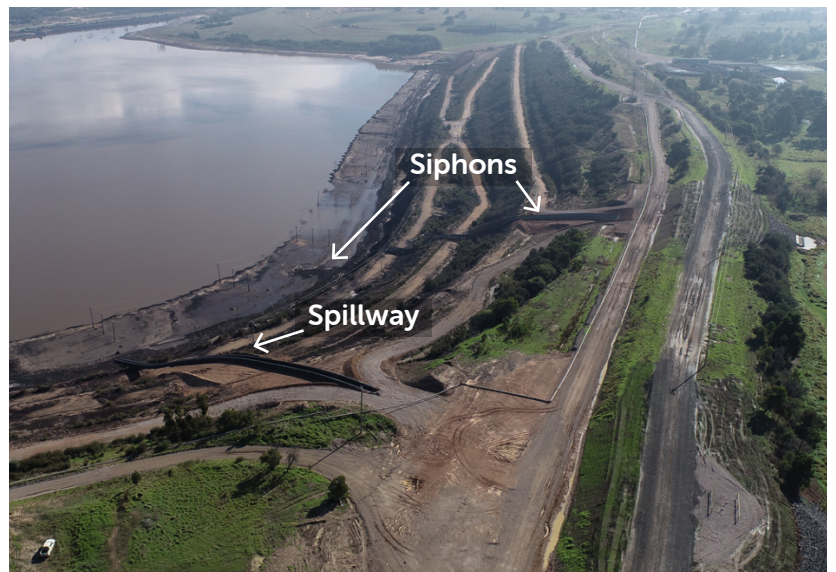
Figure 1: Aerial photo of Spillway and Siphon Location which feed water from the Morwell River to the Mine
