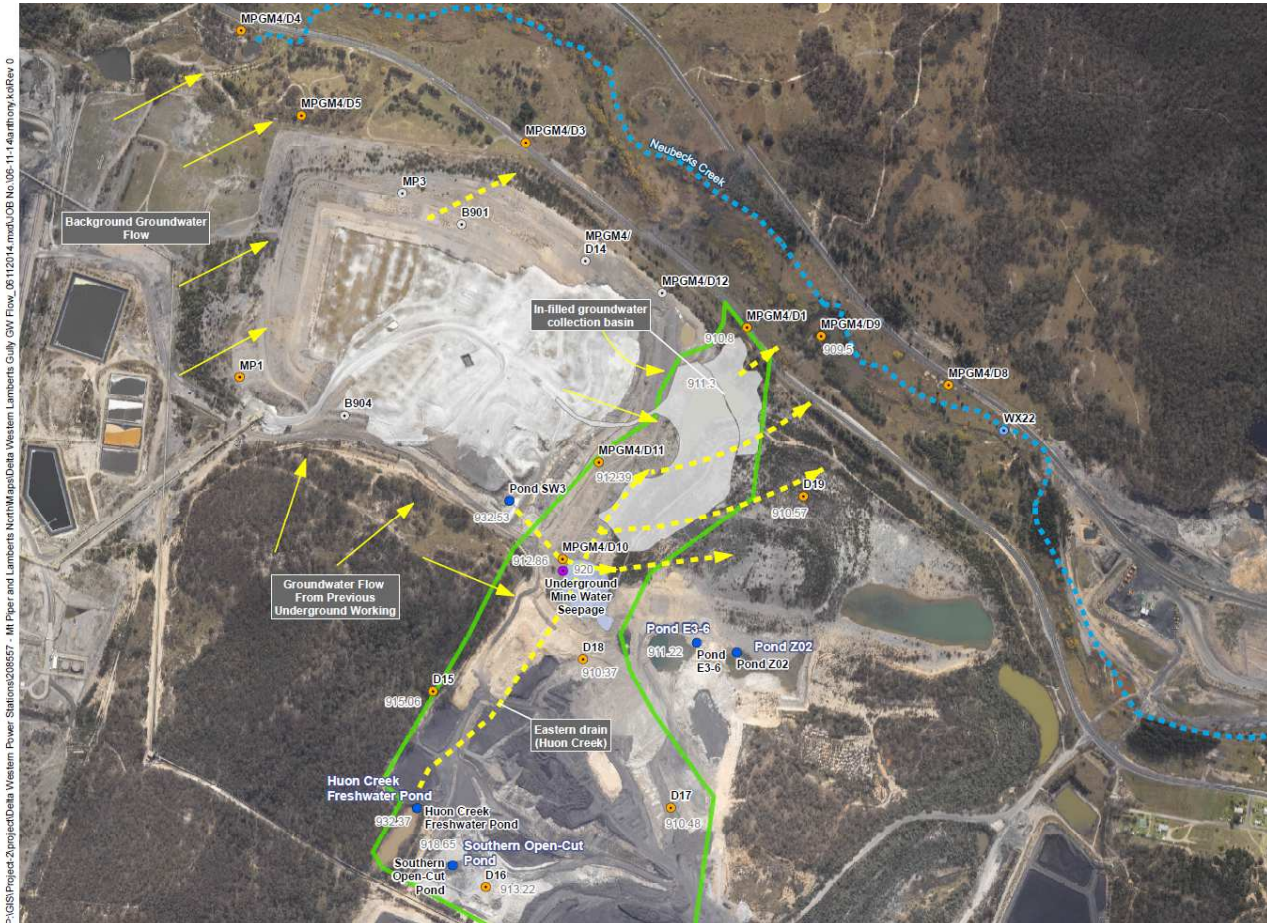
FIGURE 6: Schematic of Mt Piper Brine Co-Placement Area and Upper Lamberts North Indicative Groundwater flow paths to the in-filled Groundwater Collection Basin, bore MPGM4/D9 and Neubecks Creek
