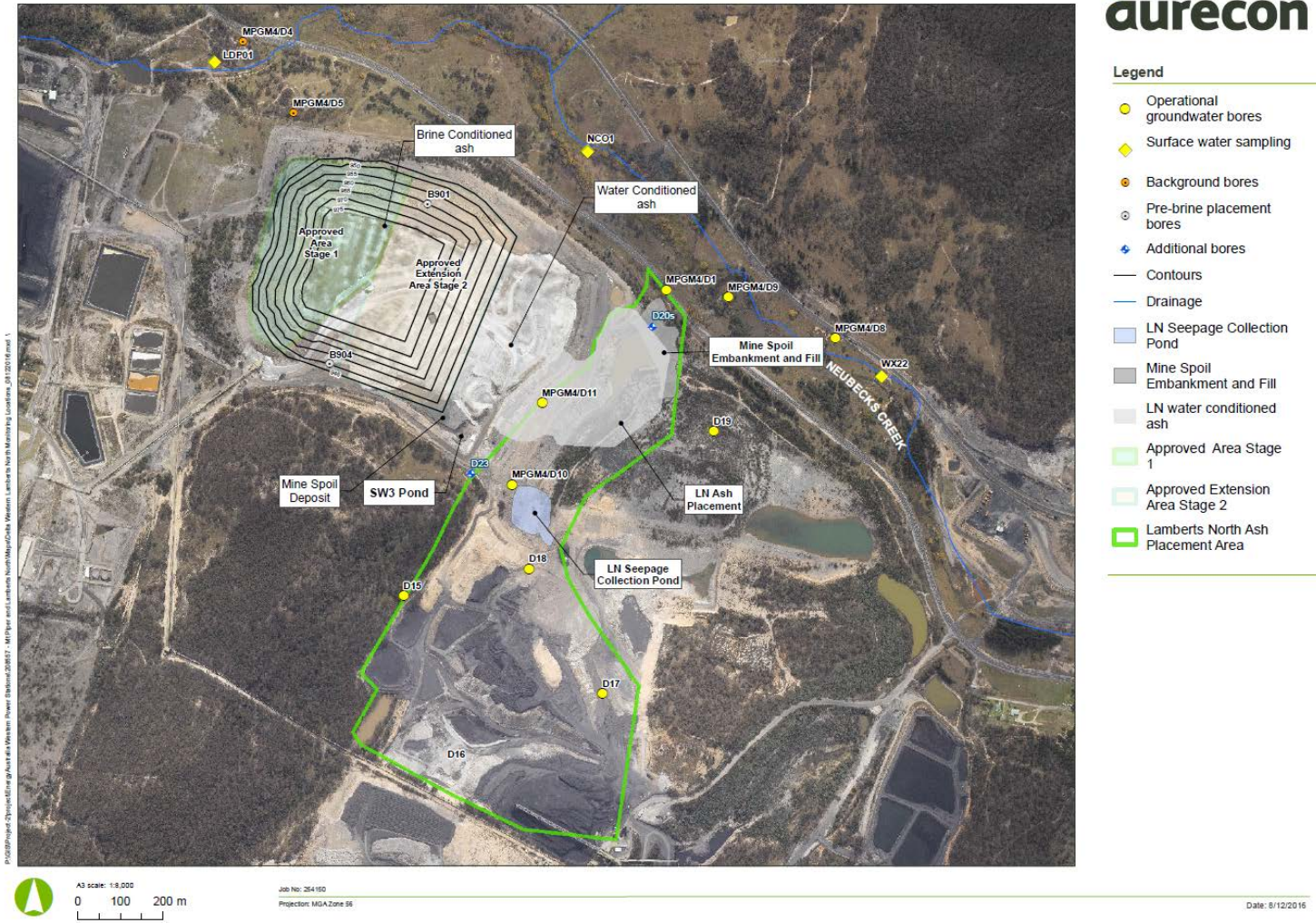
Figure 2. Lamberts North Ash Placement Area and Neubecks Creek Groundwater and Surface Water Quality Monitoring Sites
