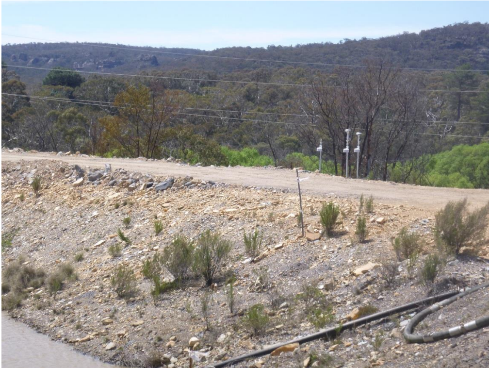
Photo 5 – Dust monitoring station - Tapered Element Oscillating Microbalance (TEOM) with vegetation screen in background
