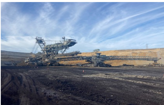
D13 and S95 link conveyor removing overburden in Maryvale Field
