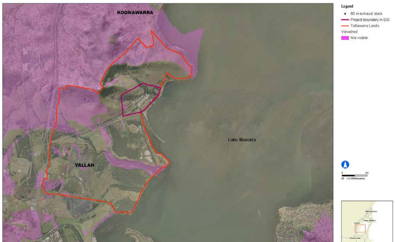
Figure 7-6 Viewshed of an exhaust stack up to 60 m high (adapted from the EIS)
