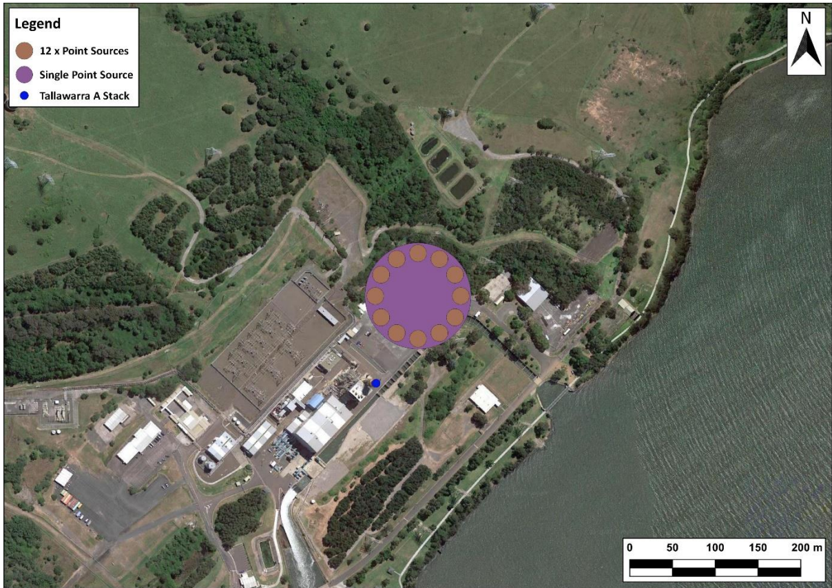
Figure A11 Modelled point source layout for the two modelling approaches of the modified PDD
